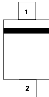
Cathode polarity for unidirectional only
